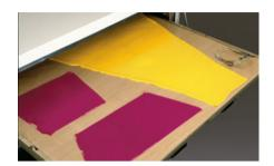
When the plastic material is heated for vacuum forming the material should sag 10-12 cm. If the material sags more than this, it will overheat and flow from the model during vacuum forming or the wall of the inner socket will become uneven and have different thicknesses.
