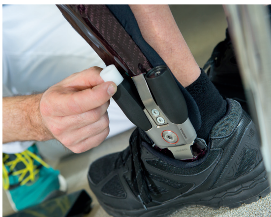
► Static alignment Insert the dummy and adjust the stop in the Reaction Module
