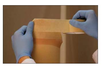
• If necessary, cover up any areas of the prosthesis that will not be sprayed using 627B6=30 Adhesive Tape.
