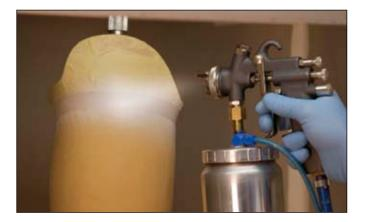
Clean the lamination resin as well as the relevant Pedilin<sup>®</sup> components (e.g., connection cap) with 634A80 Cleaning Agent and lightly apply 635C3 Primer at approximately 1.5 bar (primer does not have to be used up).
