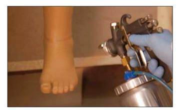
Using quick movements, spray the toe area with SuperSkin at closer range. To ensure that the toe contours remain visible, pay special attention to the recesses between the toes (as well as the space between abducted toes). Ratio of paint to air: about 50 : 50.
