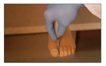
Use a curved wire (approximately 2 mm in diameter) to press on the skin created between the toes (so that the matting coat joins with the top coat and wraps around the contours of the toes.
