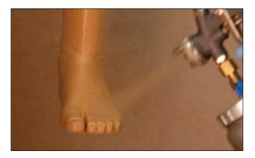
Using quick movements, spray the toe area with finish concentrate at closer range. To ensure that the toe contours remain visible, pay special attention to the recesses between the toes (as well as the space between abducted toes). Ratio of paint to air: about 50 : 50.
