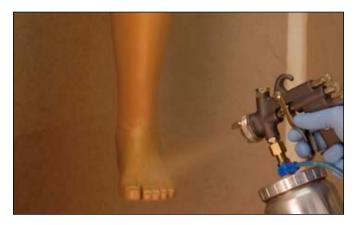
Matt the entire prosthesis with one to two coats of finish concentrate. Ratio of paint to air: about 20 : 80. **INFORMATION** Colours 1 to 7 can be matted in order to remove gloss. Colours 7 and upwards cannot be matted because otherwise a grey fog may appear.
