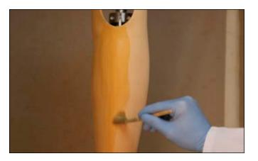
Clean laminated areas with thinner. Apply a thin lay of Otto Bock 636N9  $2 \times$  Contact Adhesive to the EVA foam or cosmetic covers wrapped in Pedilin<sup>®</sup> and let dry. This prevents overstretching of the coating material on undercuts.
