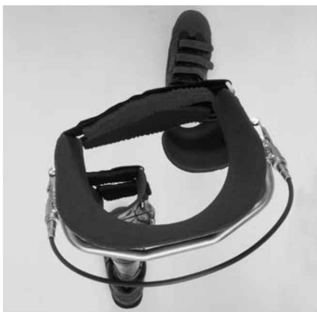
Fig. 2 At heel strike with rotated pelvis the legs remain oriented in walking direction.
